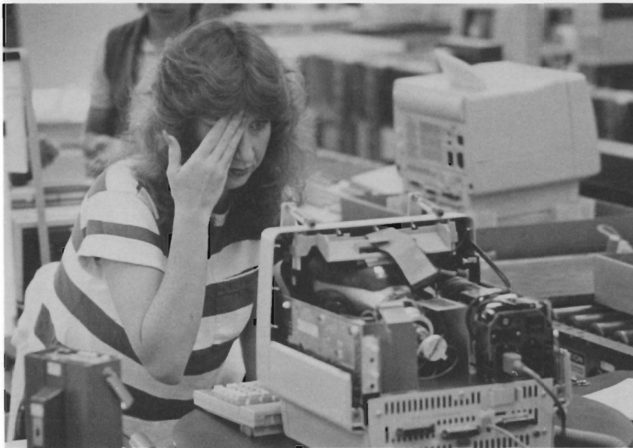
Ellen Duenas, a production worker at HP's Sunnyvale, California, facility, closes one eye to more effectively check the raster alignment of a Touchscreen personal computer.
